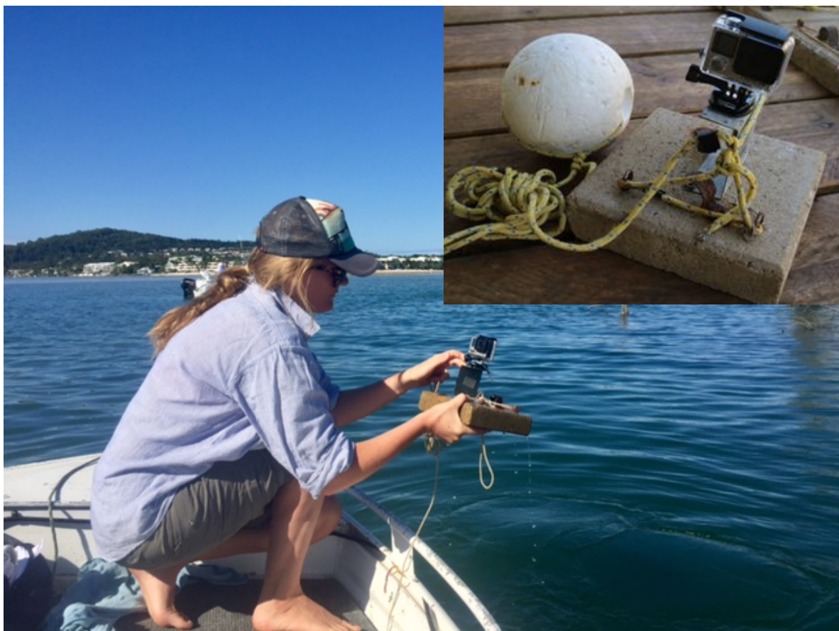
Figure 1 USC students deploying cameras to survey fish in Pumicestone Passage. Inset is the remote underwater video stations used in two parts of this project.
