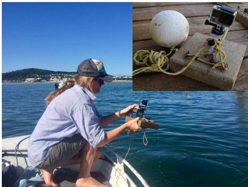
Figure 1 Deployment and design of remote underwater video stations (RUVS). BRUVS are similar in construction, but also have a length of PVC pipe which hold a crab pot bait bag containing ~500g of pilchards that attract fish to the video's field of view.
